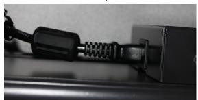
Ferrite installed on power cable
