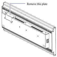
When an Alpha 9000i RGB sign is on an RS485 network, an End of Line (EOL) terminator is required at the beginning of the RS485 network and at the end of the RS485 network. The beginning of the network can be a device such as an RS232 to RS485 converter or an Alpha 9000i RGB sign. In either case, it must be terminated. The end of the network is typically an Alpha 9000i RGB sign and it should also be terminated.
