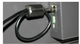
Ferrite installed on Ethernet cable
